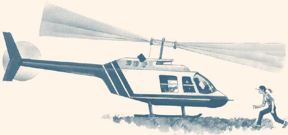
**Before approaching the helicopter, communicate with the safety personnel on the ground and come into visual contact with the pilot. Approach and leave the helicopter in a bent position, always going towards the front with your head and eyes facing forward.**
